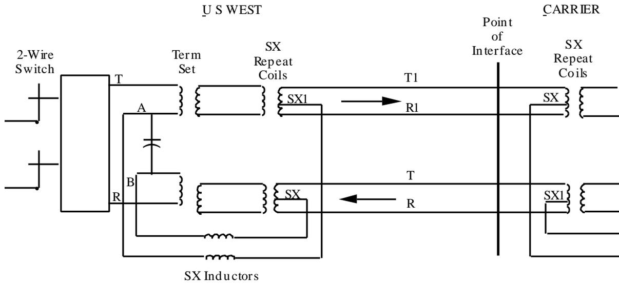
**Figure 4-3** Typical 4-Wire Configuration
