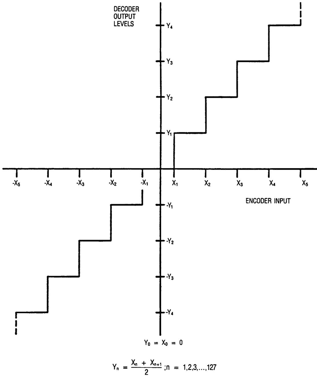
**Figure 5-7** CODEC Transfer Characteristics Information Frame
