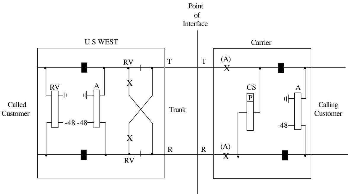
**Figure 4-2** Loop Reverse-Battery Signaling-Terminating Call
