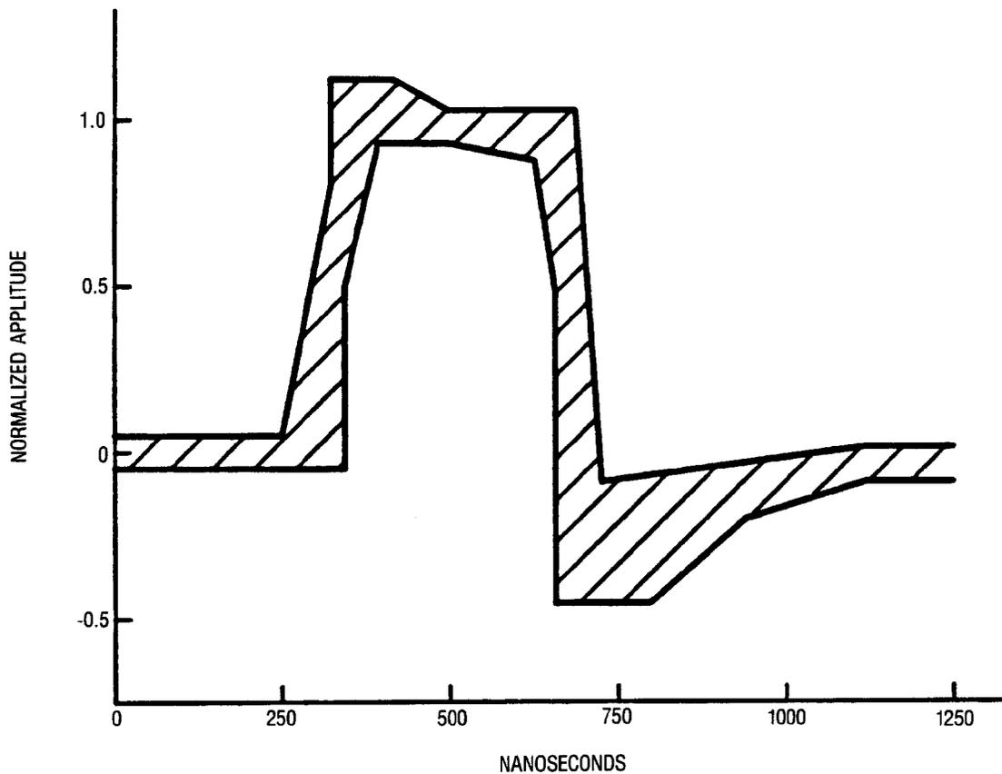
**Figure 5-2** Isolated Pulse Template For New Equipment
