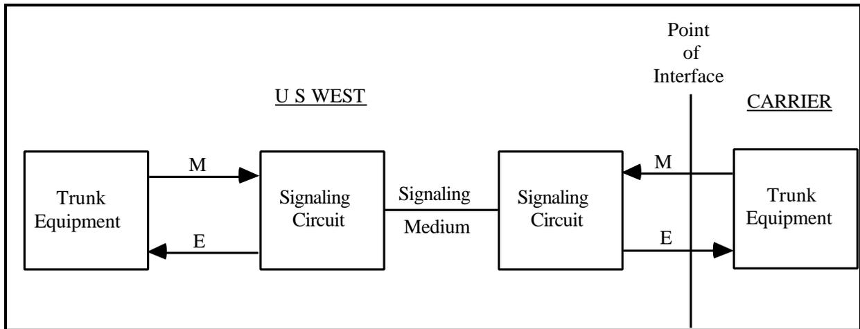
**Figure 4-4** E&M Lead Signaling
