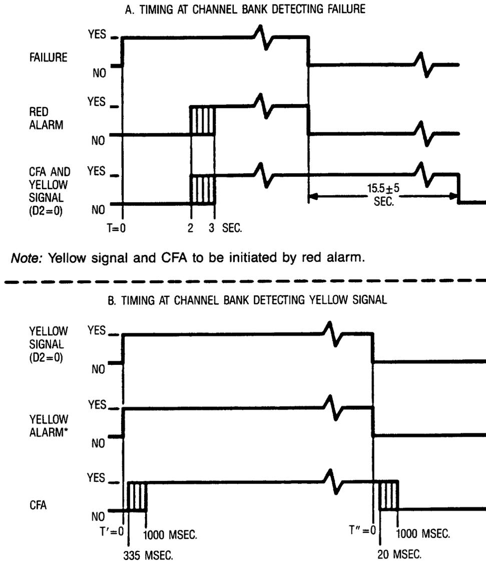
**Figure 5-5** Carrier Failure Alarm (CFA) Timing
