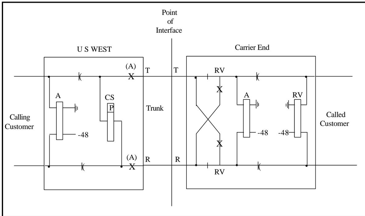
**Figure 4-1** Loop Reverse-Battery Signaling-Originating Call
