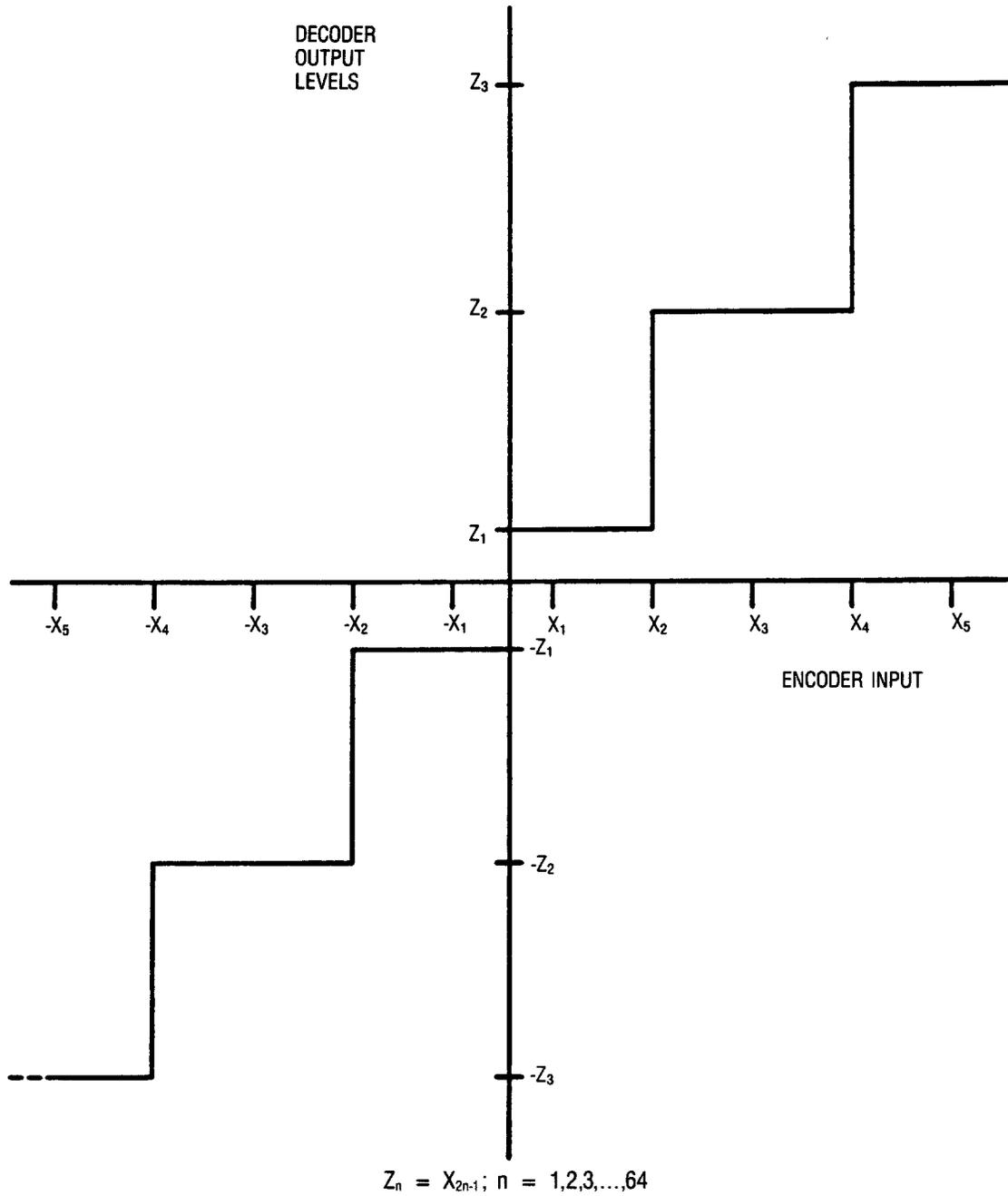
Figure 5-8 CODEC Transfer Characteristic Signaling Frame
