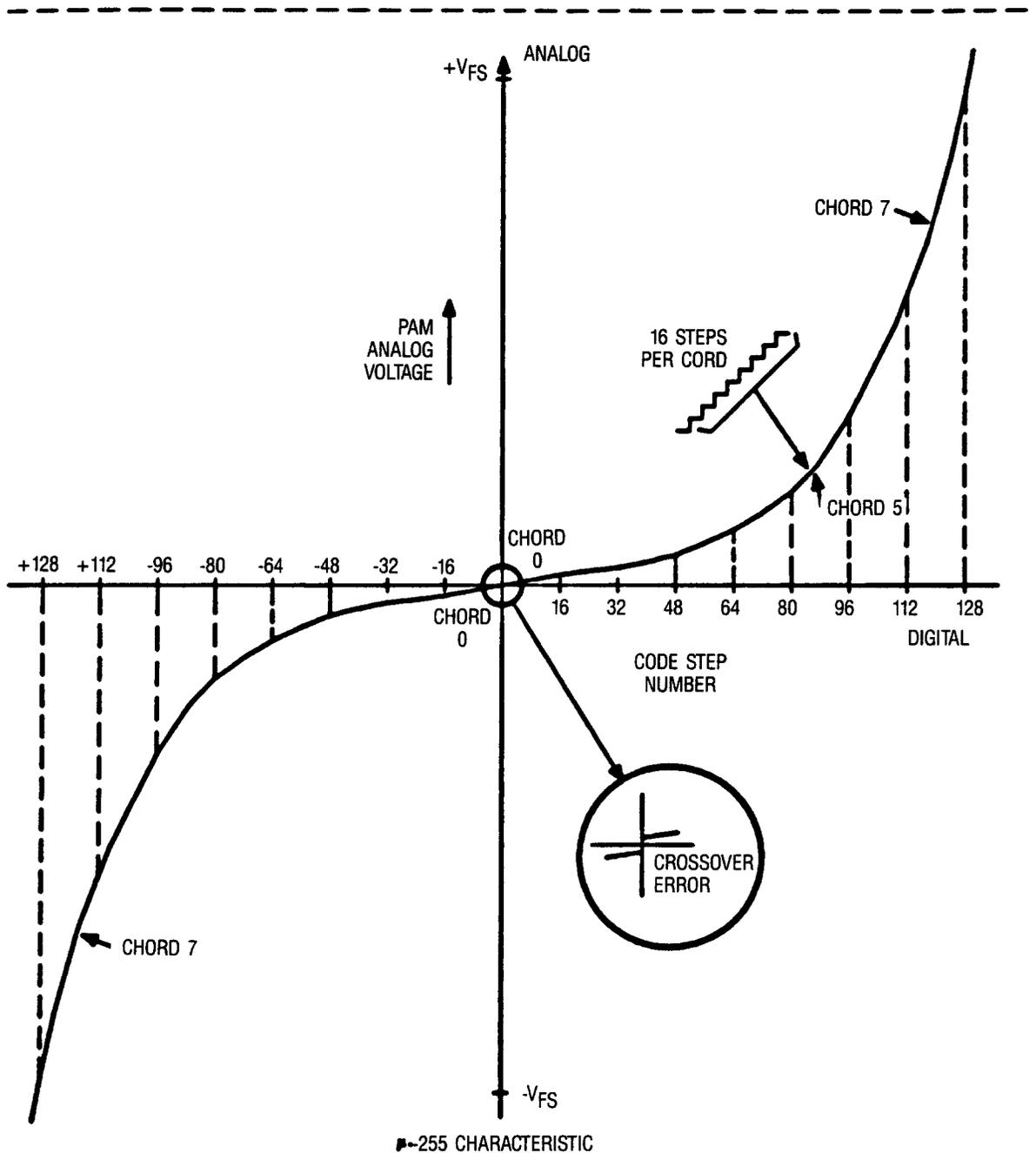
**Figure 5-6** Nonlinear Companding Characteristic of the Decoder
