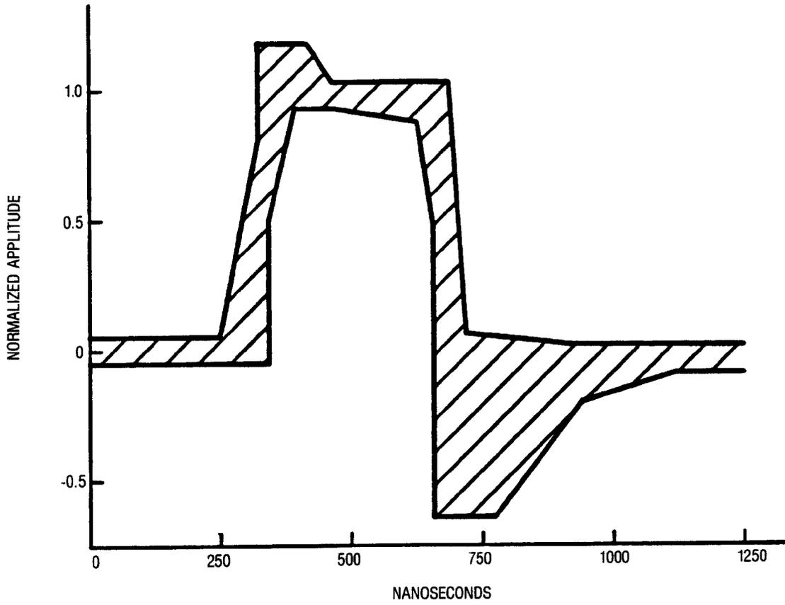
**Figure 5-3** Isolated Pulse Template For Existing Equipment
