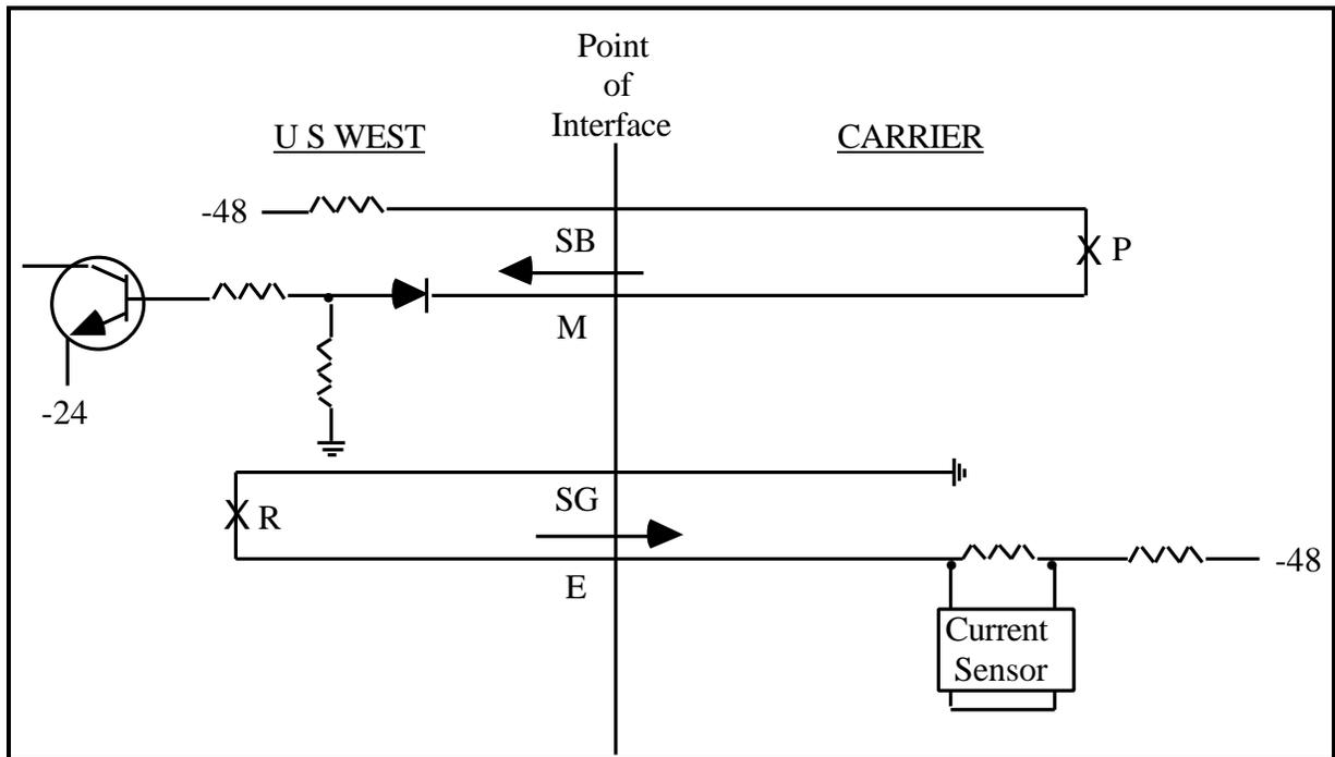
Figure 4-6 Type II E&M Lead Interface
