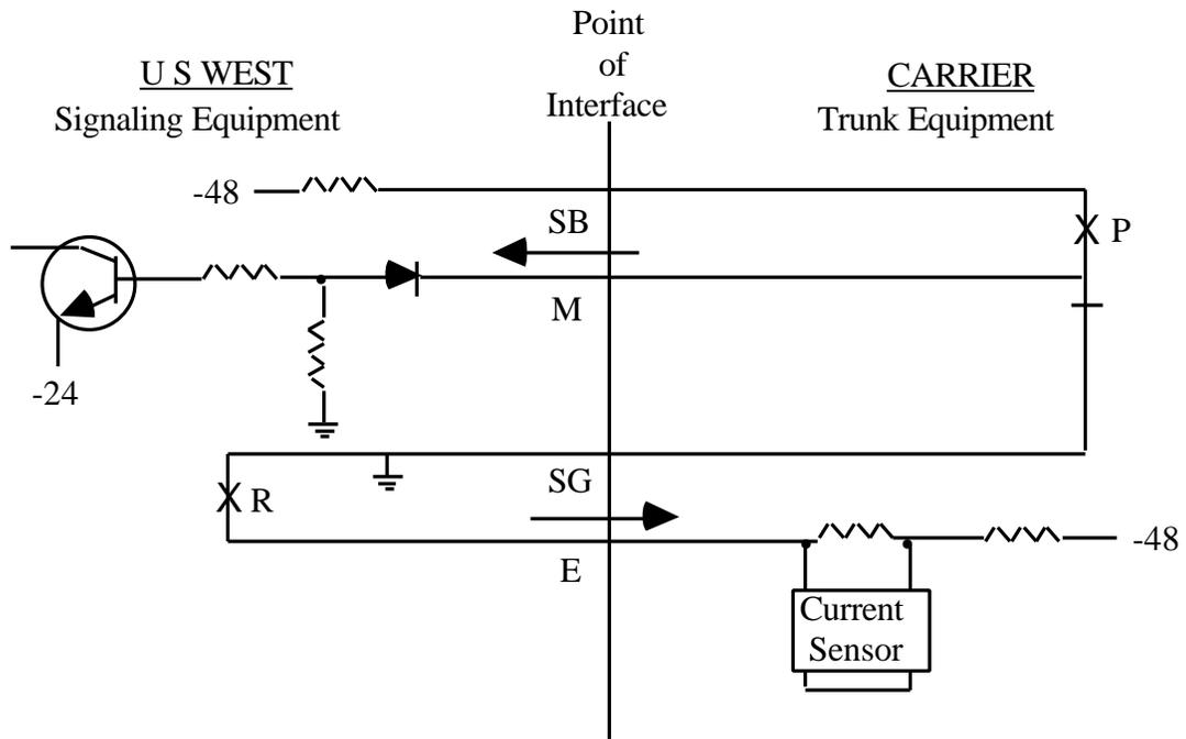
Figure 4-7 Type III E&M Lead Interface
