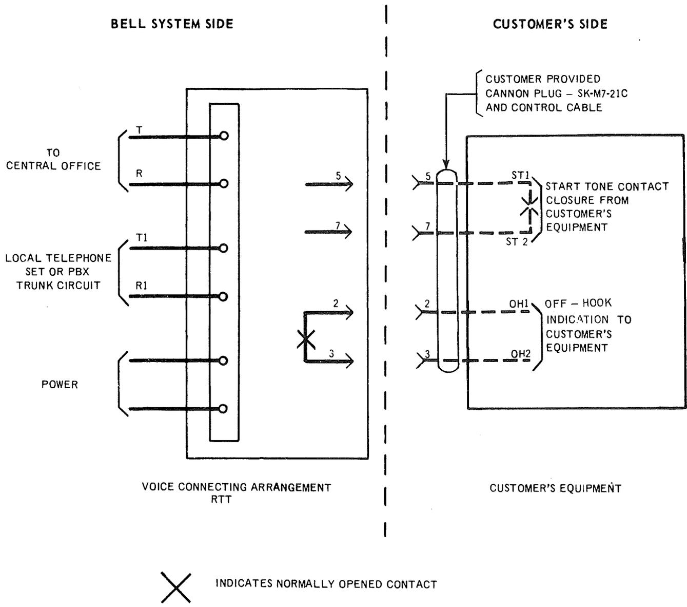
TYPICAL CONNECTIONS FOR VOICE CONNECTING ARRANGEMENT RTT
