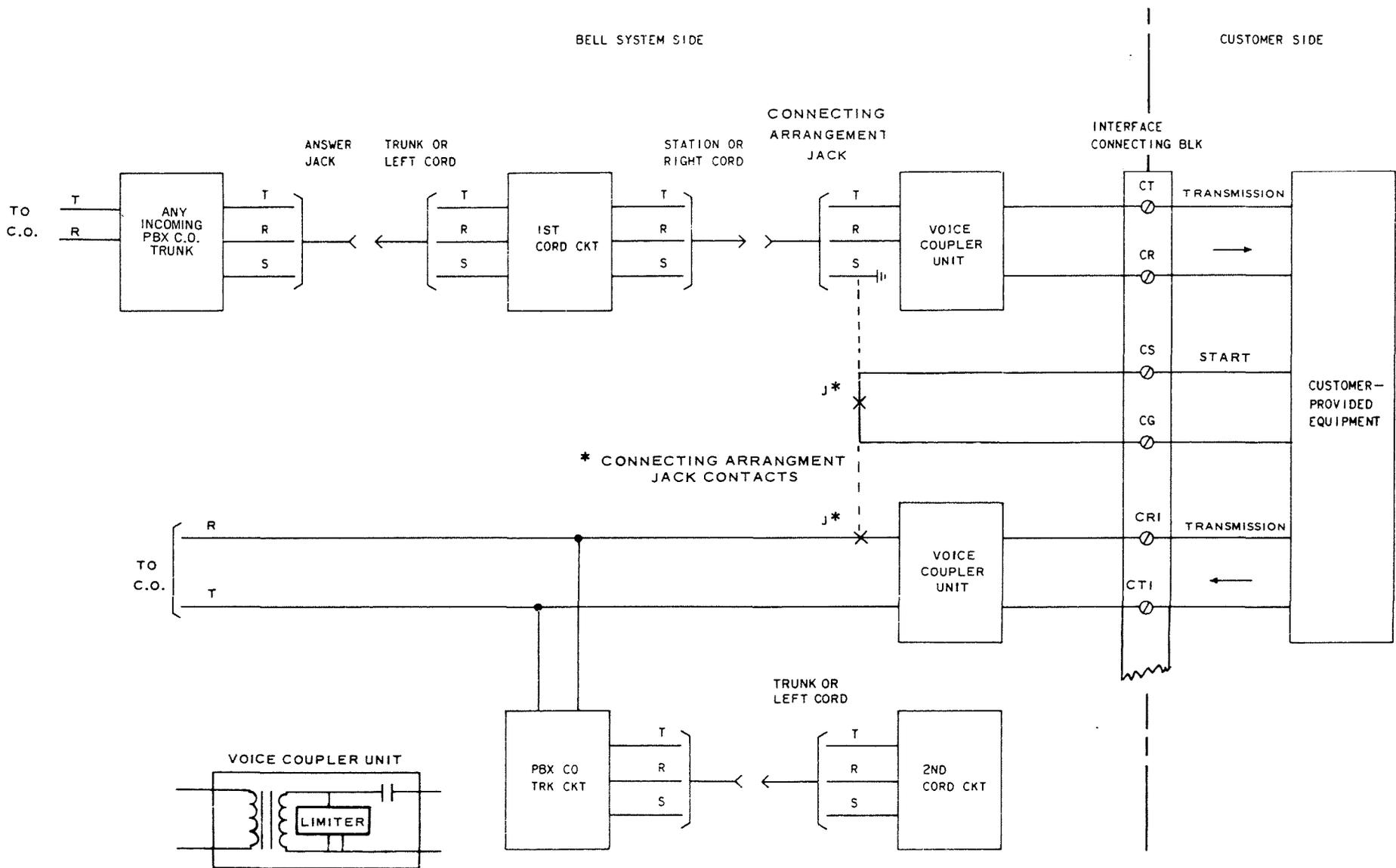
**SIMPLIFIED BLOCK DIAGRAM-VOICE CONNECTING ARRANGEMENT CDX
