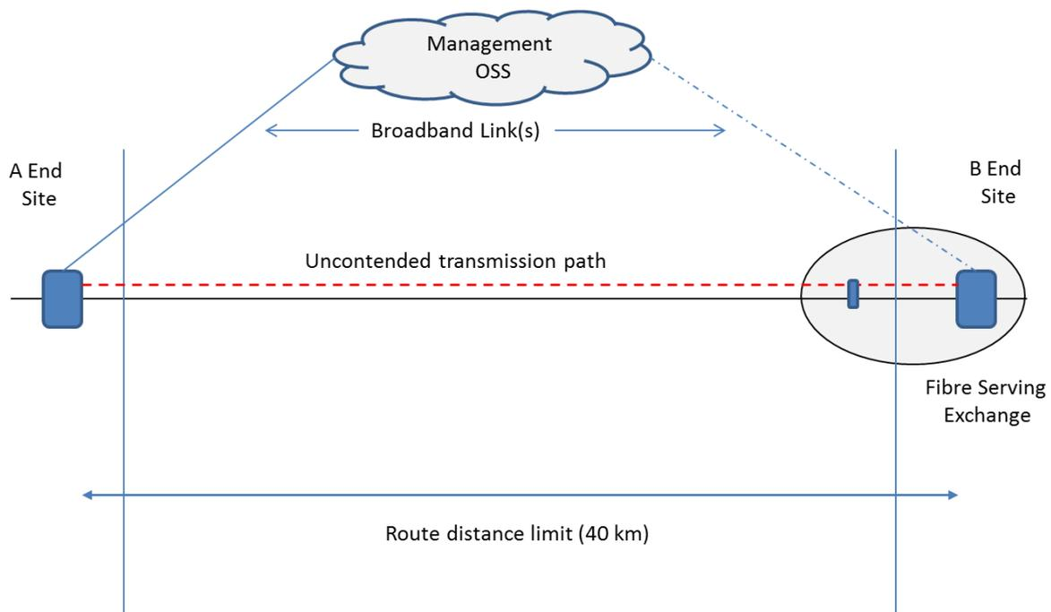
**Figure 2. EAD 10000 Local Access Service Configuration**
