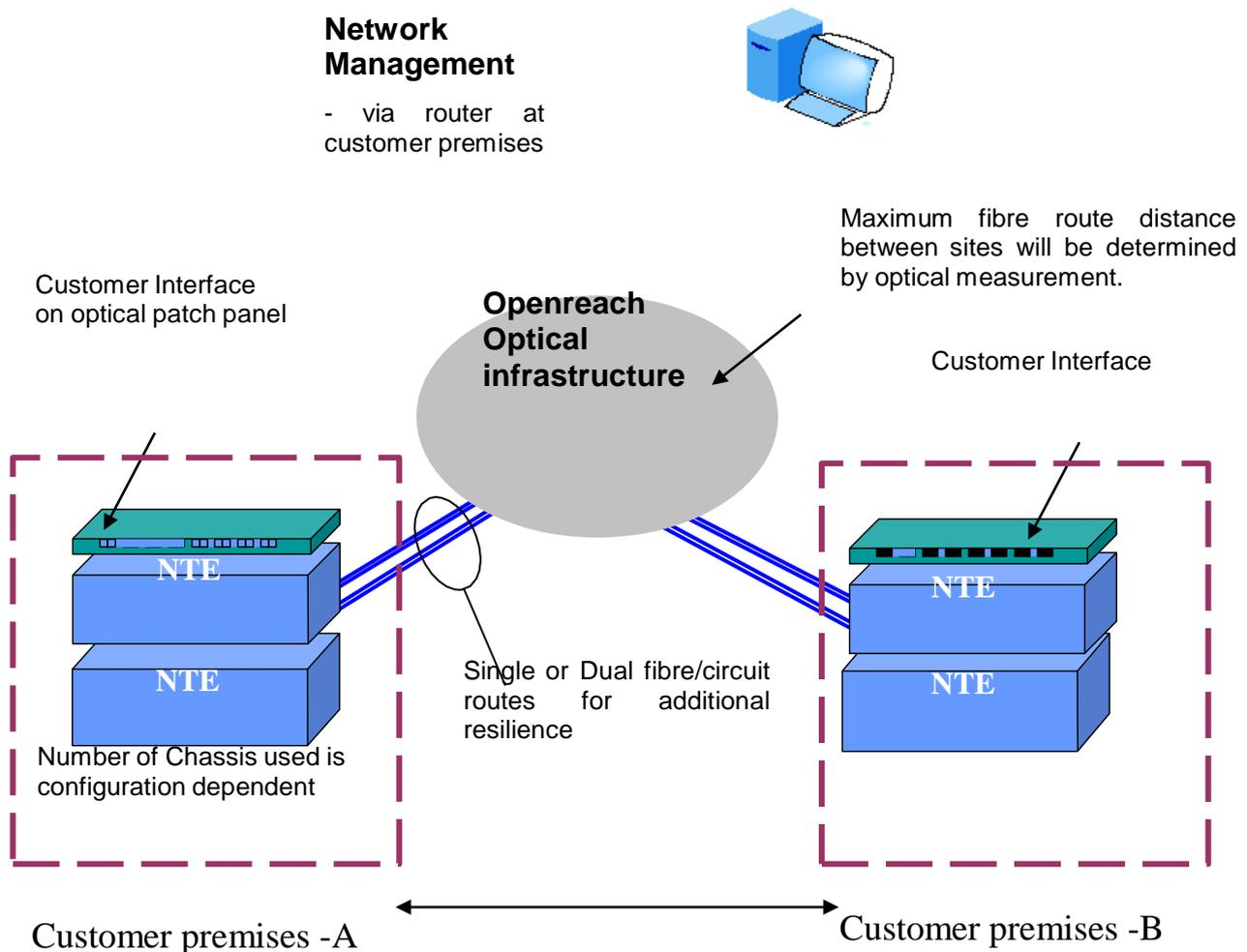
**Maximum Radial distance between BT serving exchanges is 35km for FSP2000, There is no Maximum distance on FSP 3000 but both are dependent on fibre route distance and card/filter configuration.**
