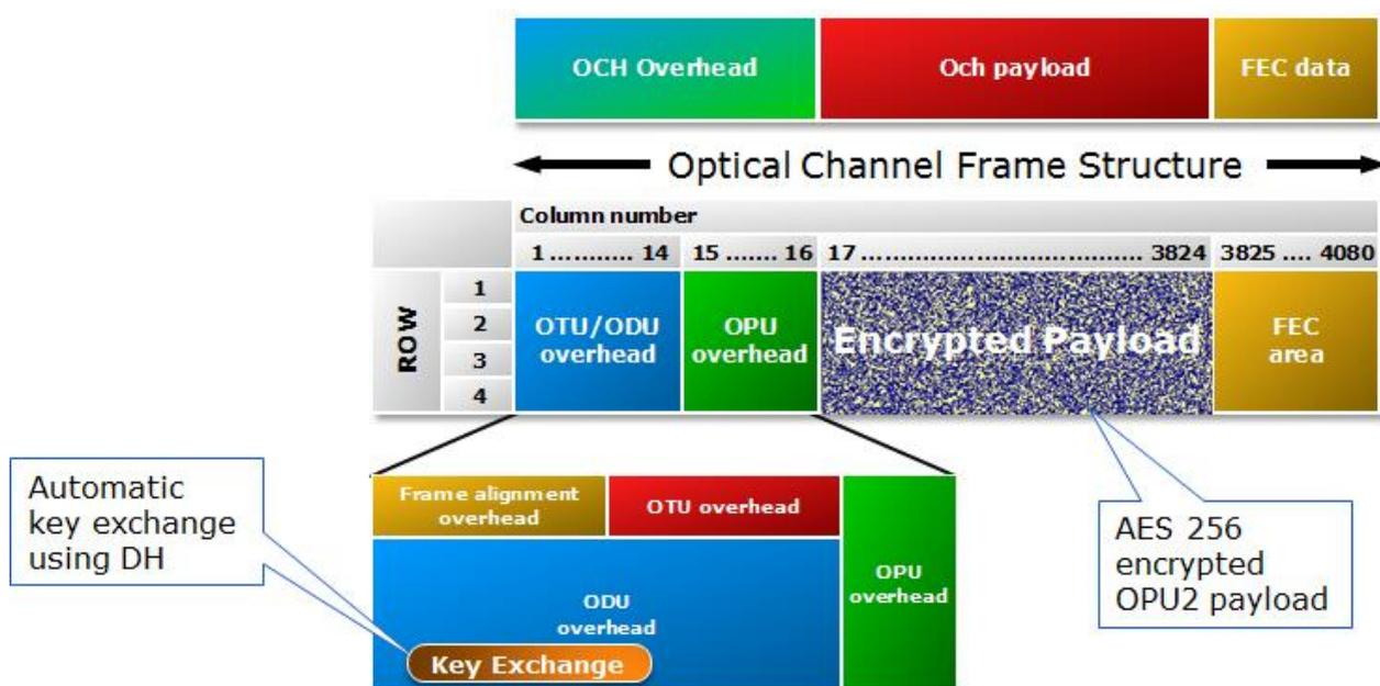
The 5TCE-PCTN-10G-AES card is built around symmetric-key encryption standard Advanced Encryption Standard AES256 announced by the National Institute of Standards and Technology (NIST). The encryption solution utilises Diffie Hellman key exchange and a dedicated Openreach security NOC team.
