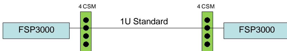
A single 4-channel filter (4CSM) is fitted as standard to this bearer, therefore this service will support (non-traffic affecting) channel growth to 4 wavelengths.
