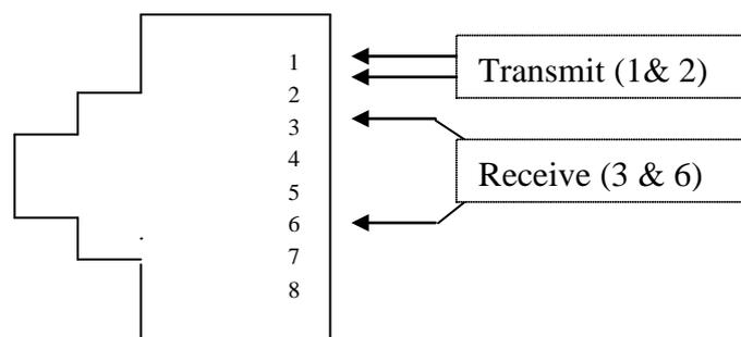
*Figure 2. BES 100 NTE RJ45 Connector Pin Out Connections*
