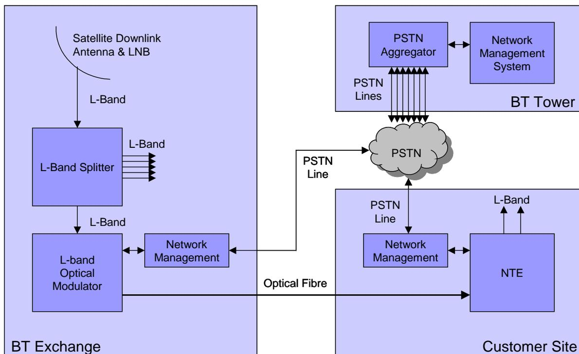
**Figure 1 System Diagram**
