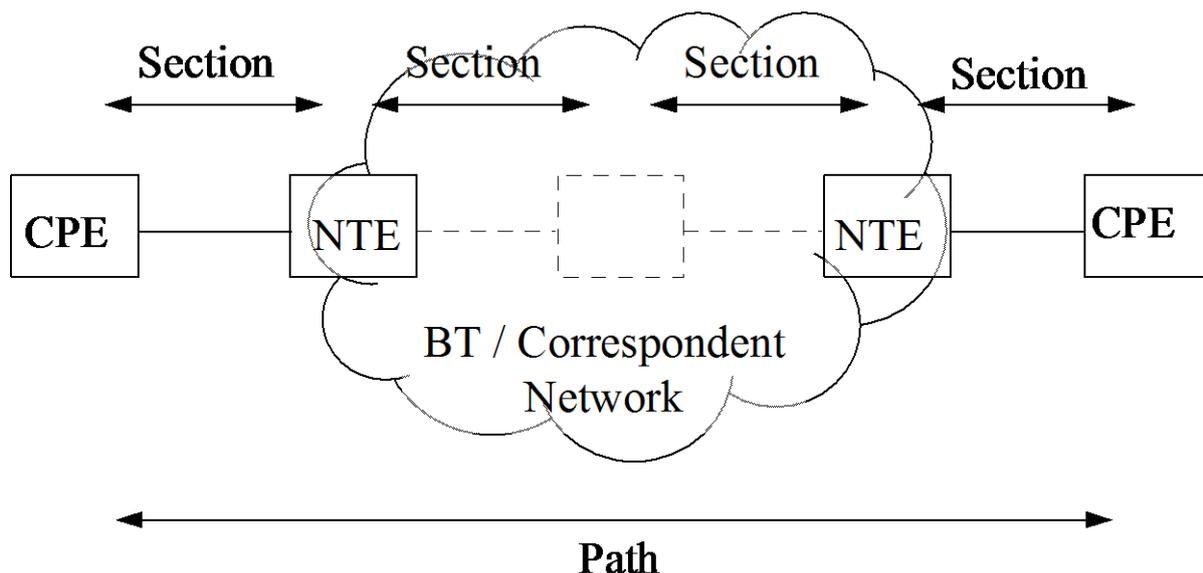
**Figure 1 - Comparison of SDH Path vs. Section**
