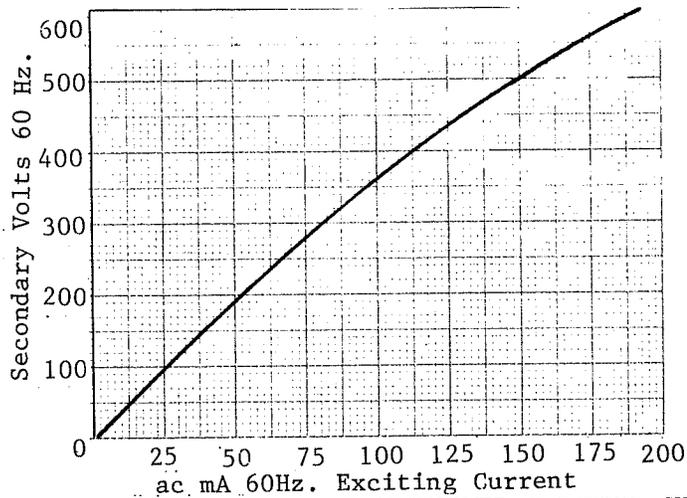
FIGURE 2: NEUTRALIZING TRANSFORMER EXCITING CURVE
