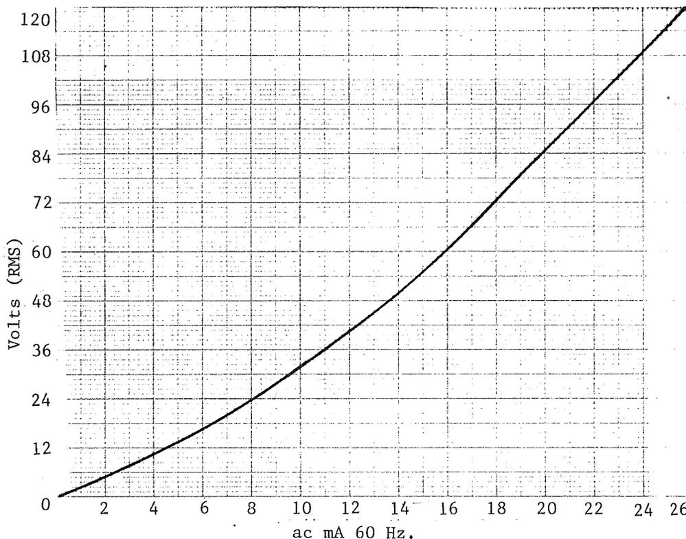
FIGURE 1: NEUTRALIZING TRANSFORMER (EXCITING CURVE)
