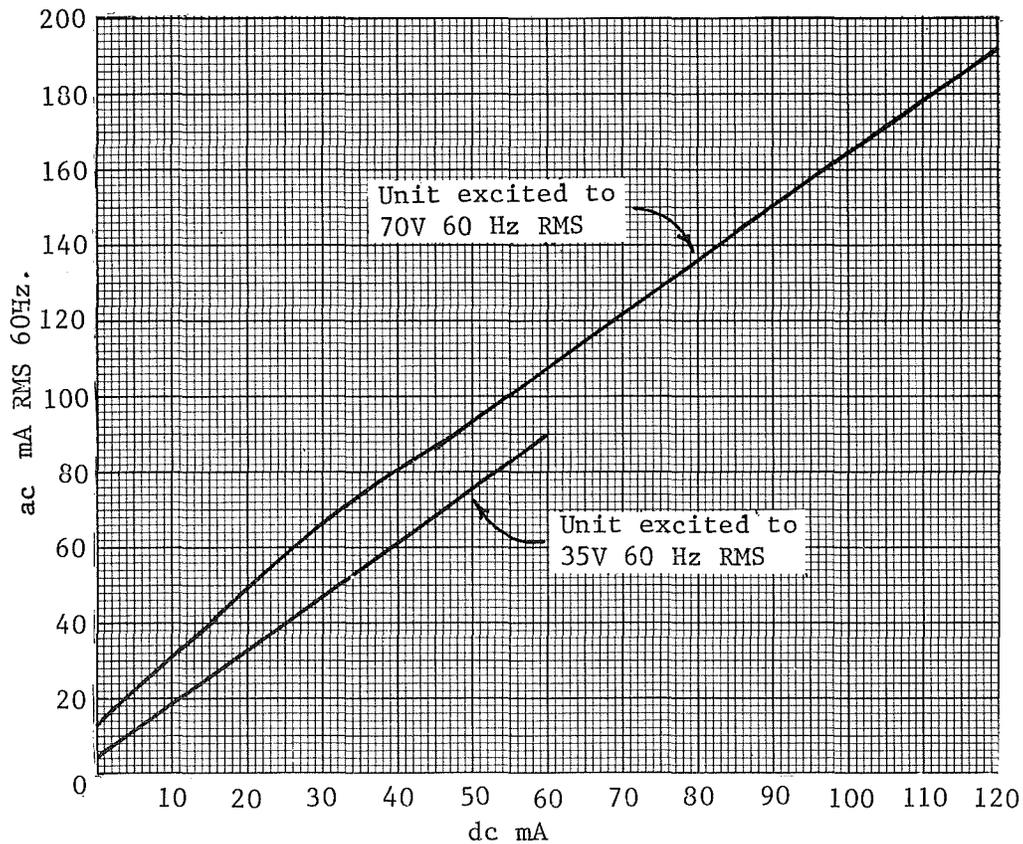
FIGURE 3: LONGITUDINAL NOISE CHOKES (EFFECT OF DC CURRENT)
