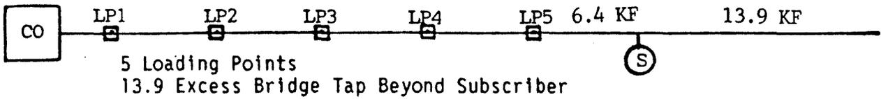
Loop F: 23.0 KF, 22 Gauge, D66 Loaded
