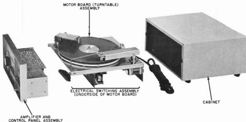
Figure 2. Model SP-2: Principal Assemblies.
