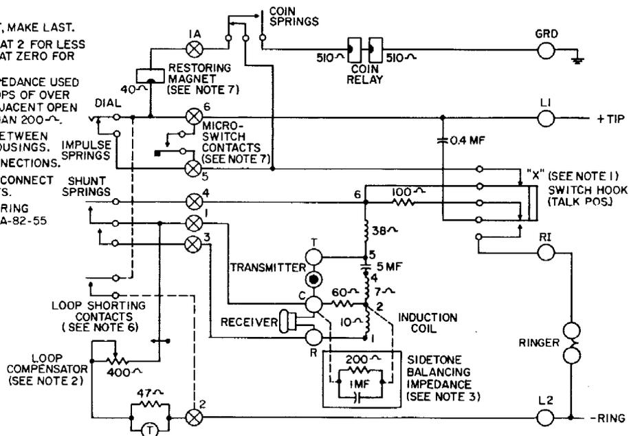
Figure 14. Type LPA-82 Prepay Paystation - Schematic Diagram
