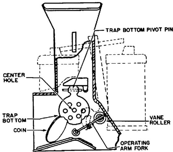
Figure 6. Trap and Vane in Refund Position
