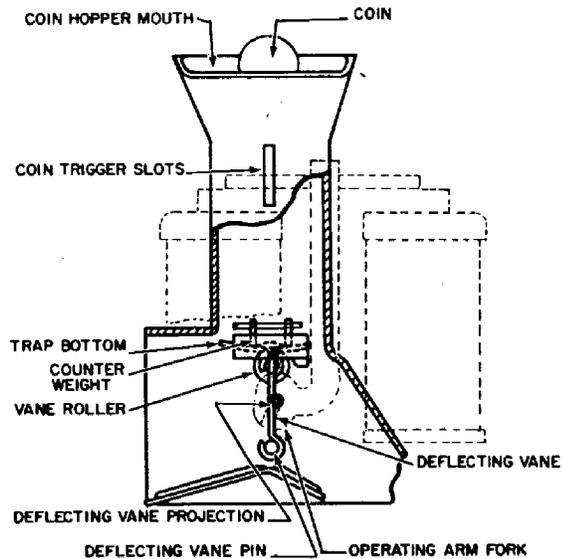
Figure 5. Trap and Vane in Normal Position
