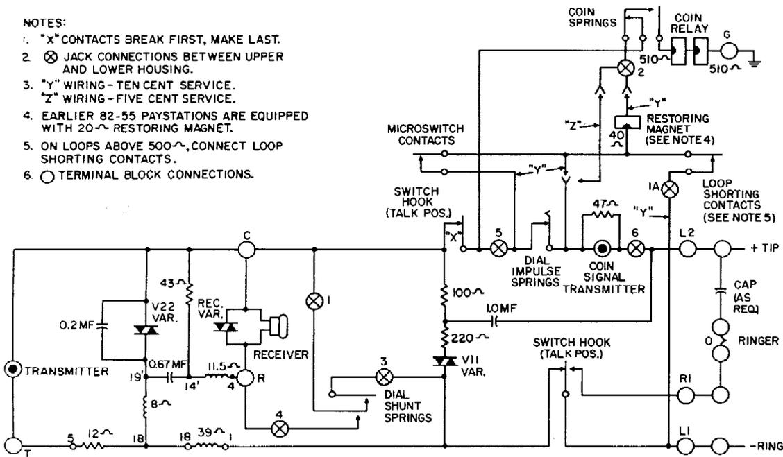
Figure 15. Type LPB-82 Prepay Paystation - Schematic Diagram
