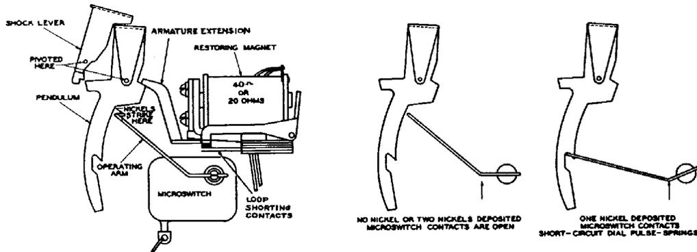
Figure 3. Two-Nickel Assembly
