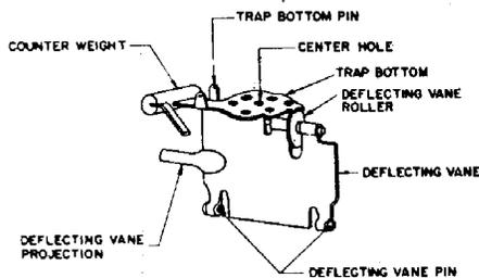
Figure 4. Coin Hopper Trap and Vane Assembly
