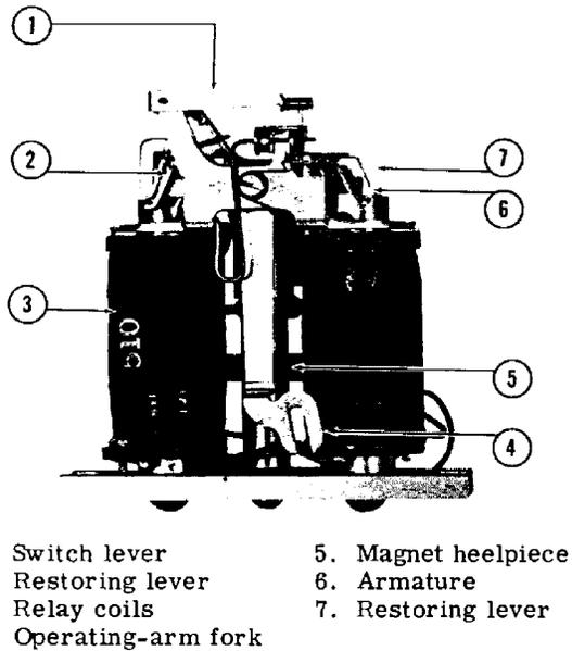
Figure 8. Coin Relay (Rear View)
