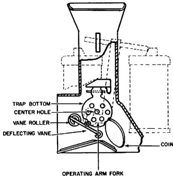
Figure 7. Trap and Vane in Collect Position
