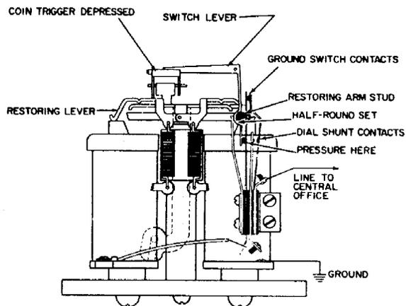
Figure 10. Coin Relay - Coin Trigger Tripped
