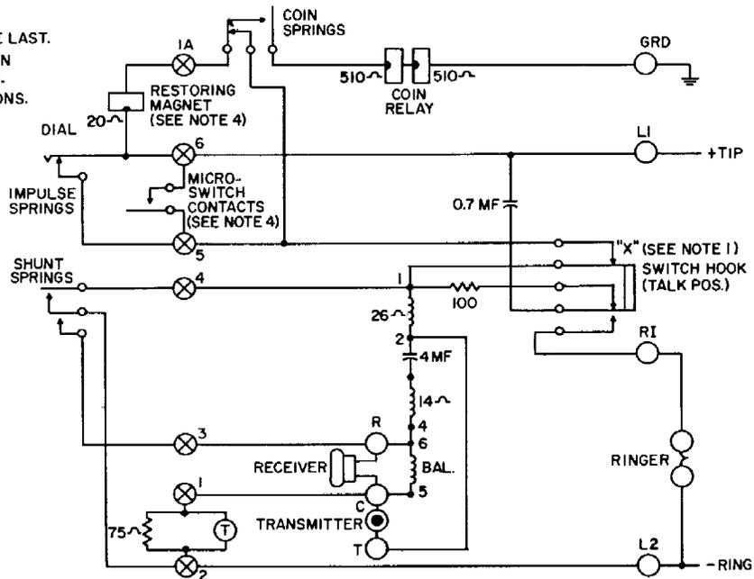
Figure 13. Type 62 Prepay Paystation - Schematic Diagram
