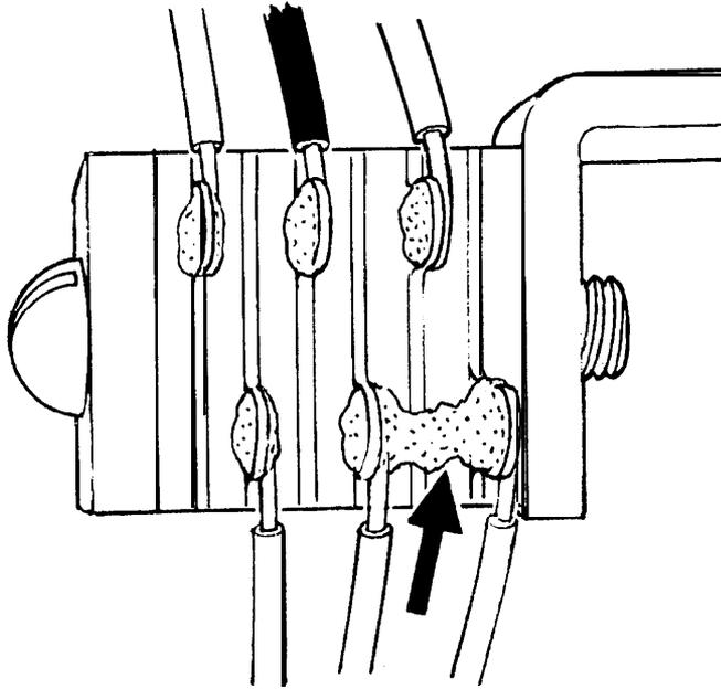
Figure 13. Solder Bridge or Short
