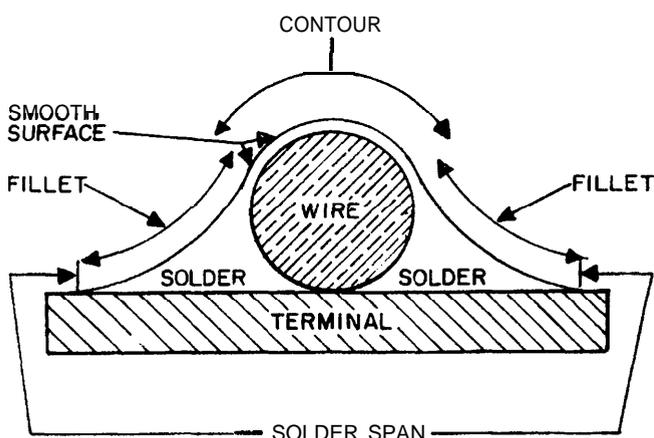
Figure 9. Characteristics of a Good Soldered Joint.
