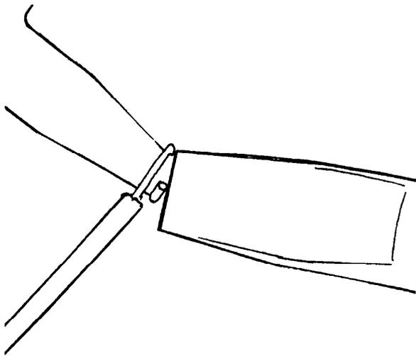
1. CAREFULLY POSITION THE IRON ON THE CONNECTION, WITH AS MUCH CONTACT AS POSSIBLE. AVOID TOUCHING THE INSULATION.
