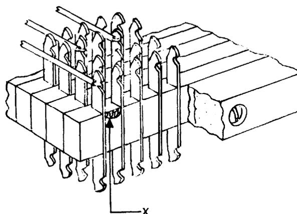
Figure 12. Excessive Solder Causing Cross "X" Short
