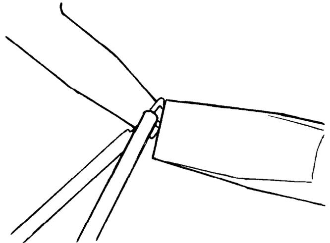
2. APPLY SOLDER TO THE CONNECTION. FEED ONLY ENOUGH TO COVER THE CONNECTION.
