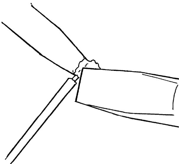
3. WITHDRAW SOLDER ONLY. WITH THE IRON ON THE CONNECTION, WATCH FOR PROPER SOLDER FLOW.
