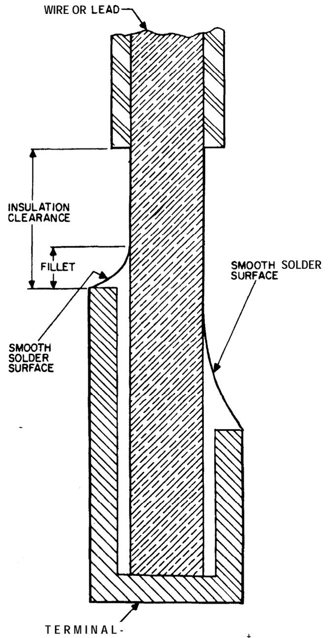
Figure 19. Characteristics of a Good Soldered Joint for a Cut-Away Tubular Terminal.
