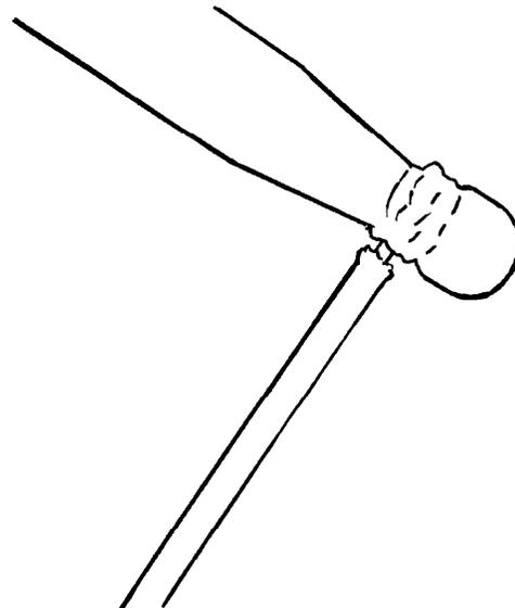
4. WITHDRAW THE IRON WITH A WIPING MOTION TO SMOOTHLY COVER THE WIRE AND REMOVE ANY SURPLUS SOLDER.
