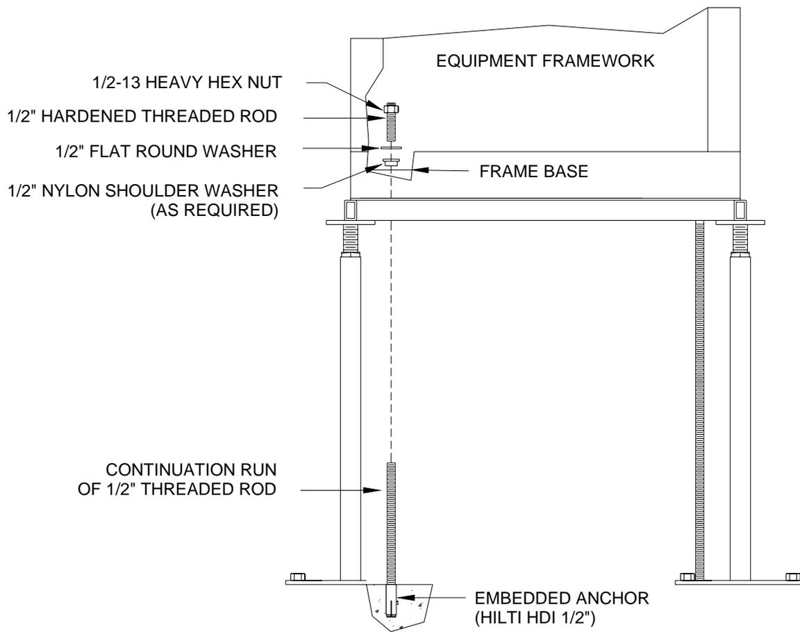
**FIGURE 14. Floor Channel Anchoring Method**
