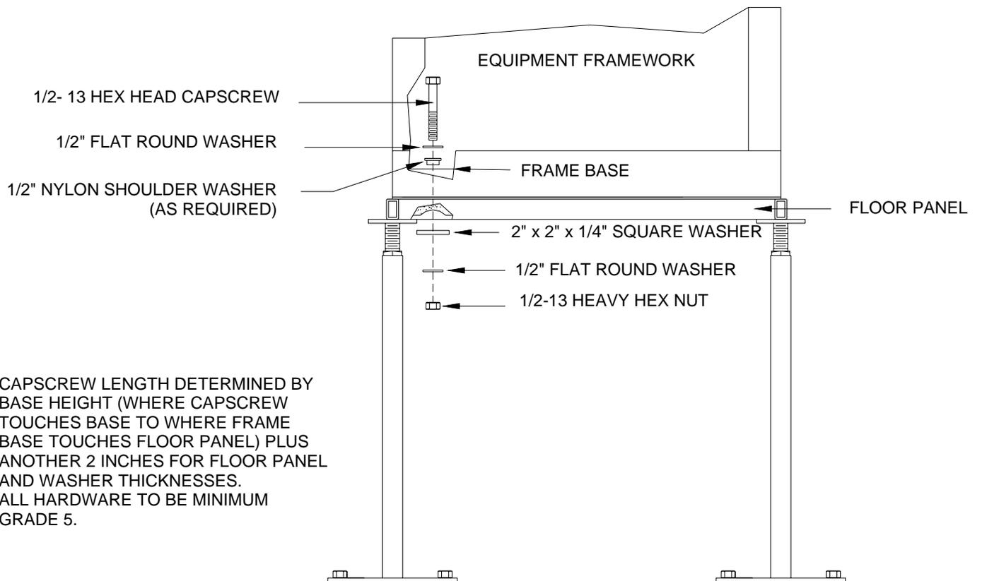
**FIGURE 18. Panel Underside Washer And Nut Assembly**
