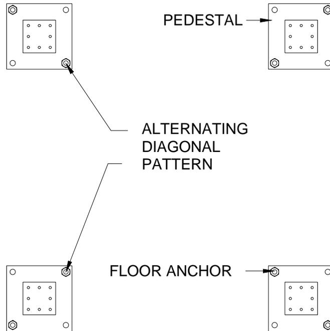
**FIGURE 9. Access Floor Grounding Grid**
