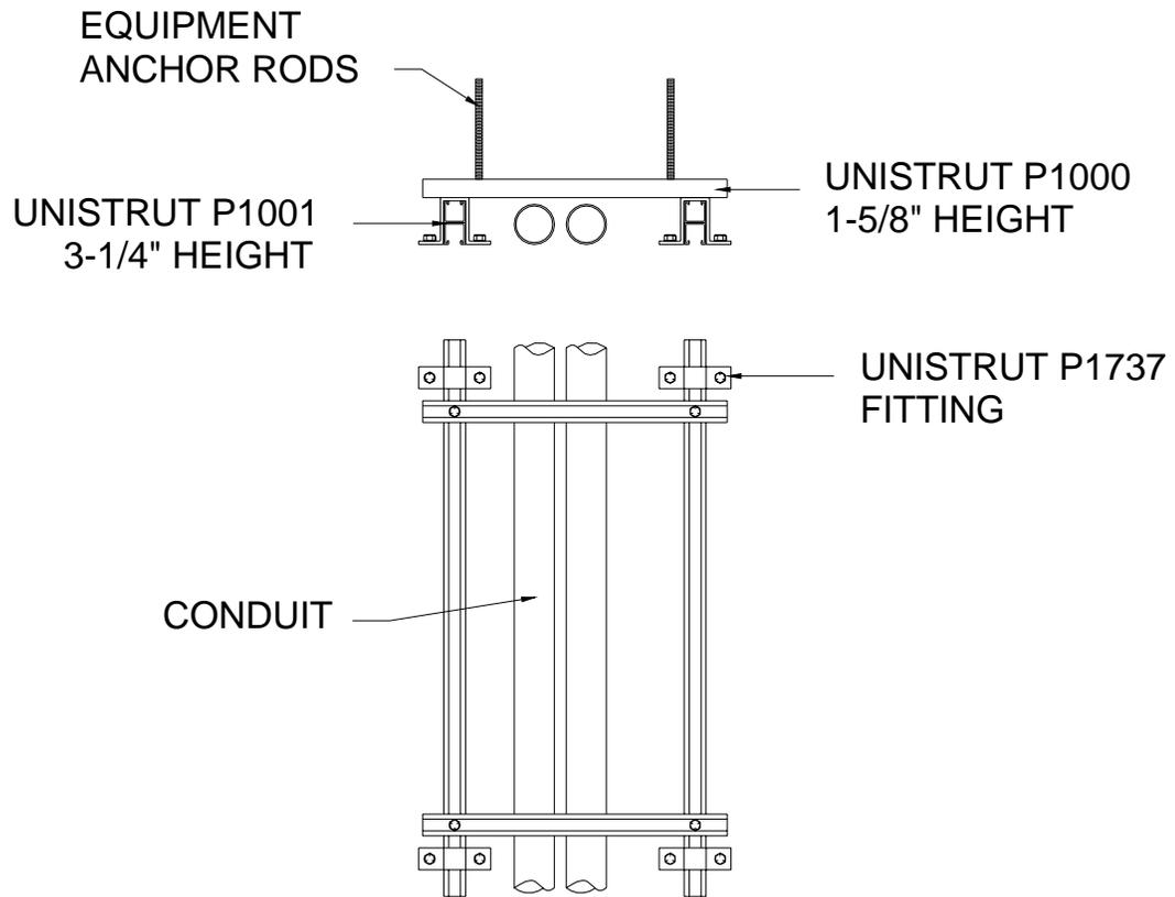
**FIGURE 16A. Cross Aisle Bracing**
