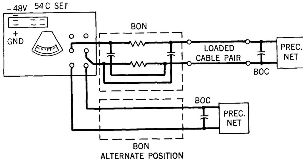
Circuit for Return-Loss Measurements
