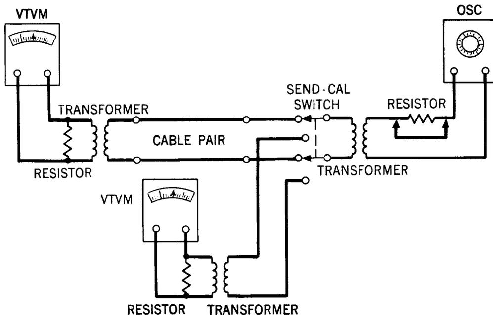
Circuit for Transmission-Loss Measurements
