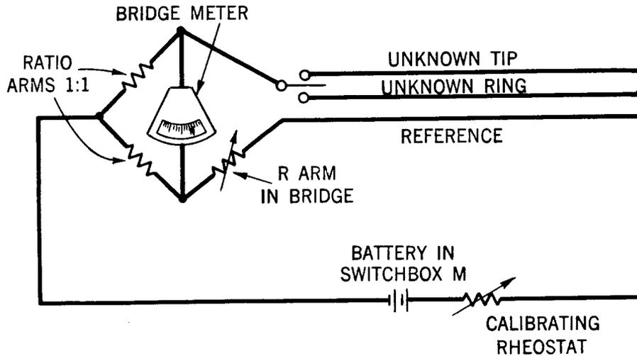
Circuit for Resistance Measurements
