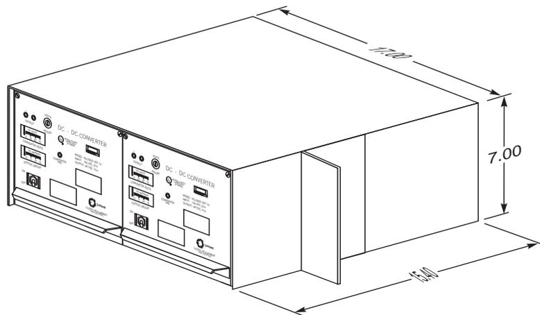
**Figure 1-1: DC-DC Converter Shelf Assembly
