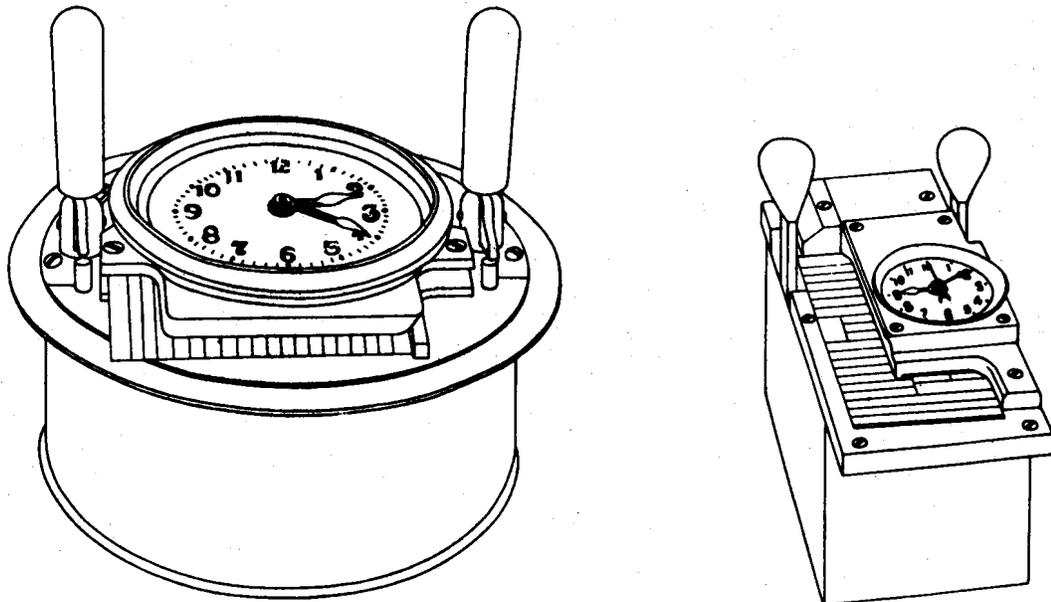
Fig. 1 - Electrically Driven Calculagraphs.
