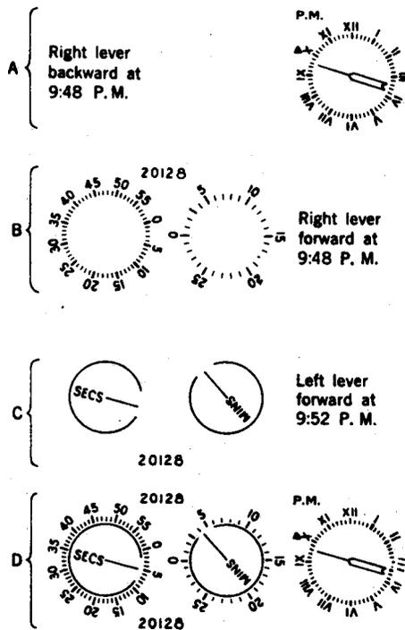
Note: Impressions designated by A and B are made at the start of conversation and that designated by C at the end of conversation. D shows the completed impression as it appears on the ticket to indicate the elapsed time of 4 minutes and 5 seconds starting at 9:48 P.M.
