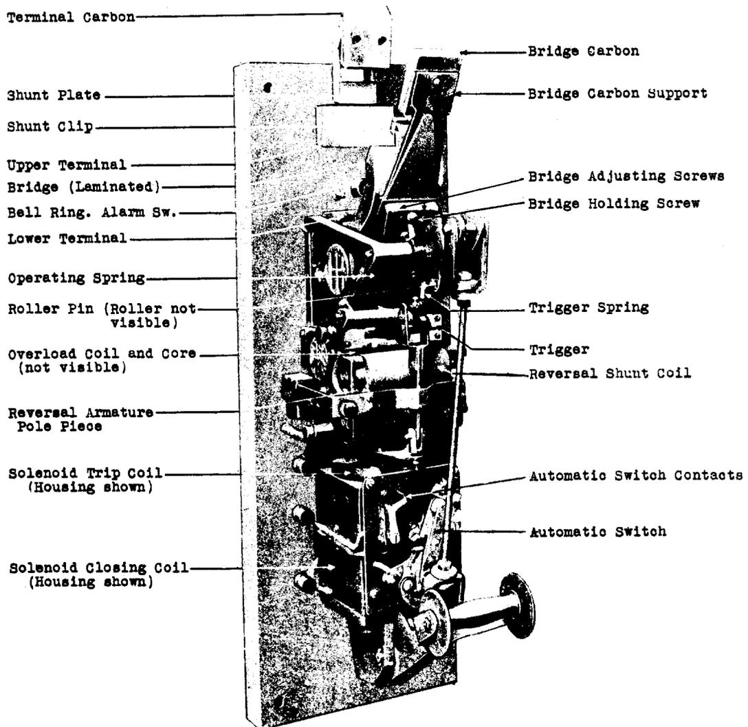
Fig. 1 - Type LL Breaker - Solenoid Operated
