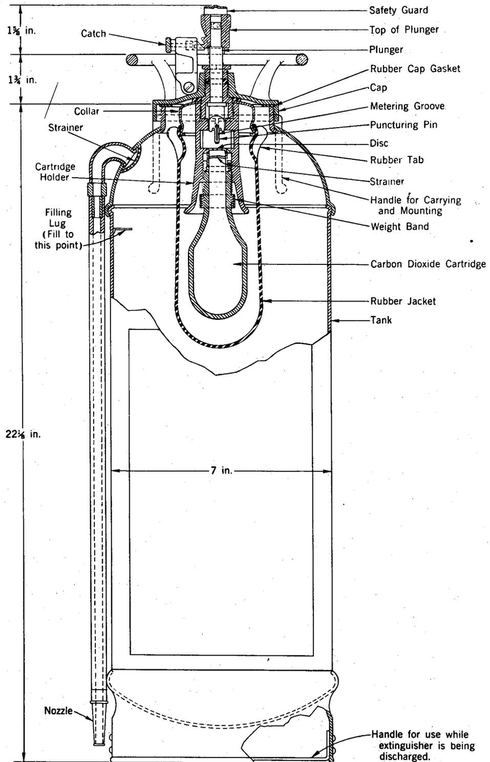
Fig. 4 - Water Extinguisher - Newer Design
