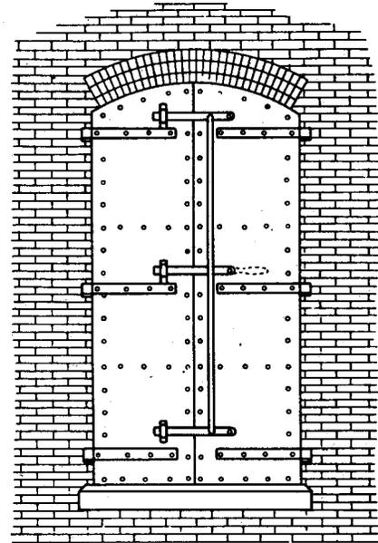
Fig. 10 - Manually Operated Fire Shutter - Closed
