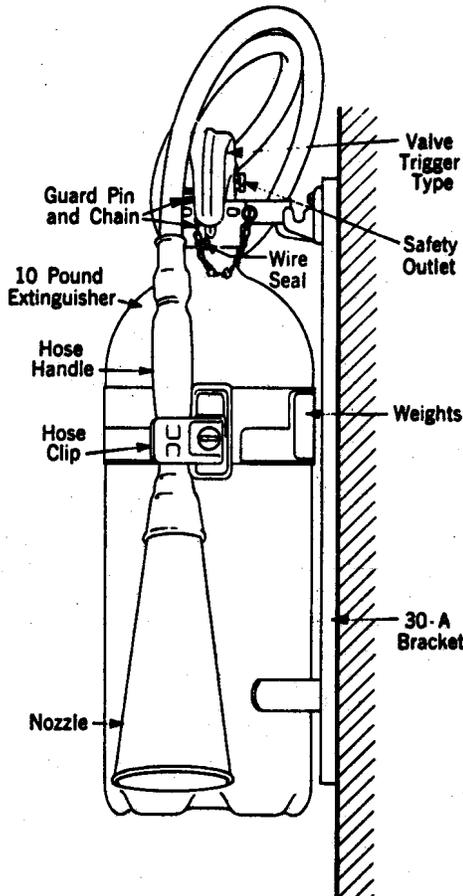
Fig. 1 - Carbon Dioxide Extinguisher - Newer Design
