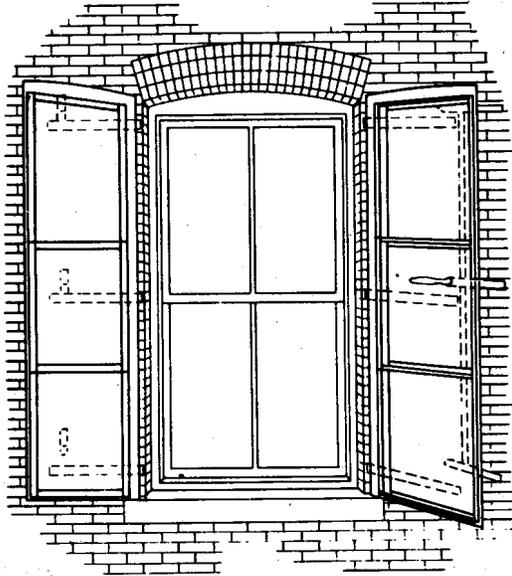
Fig. 9 - Manually Operated Fire Shutter - Open
