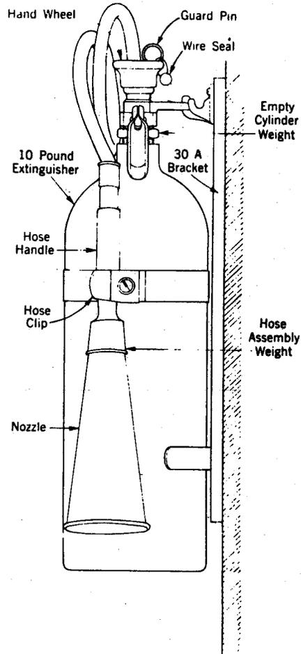
Fig. 2 - Carbon Dioxide Extinguisher - Former Design
