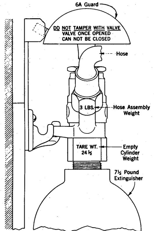
Fig. 3 - Handwheel Guard
