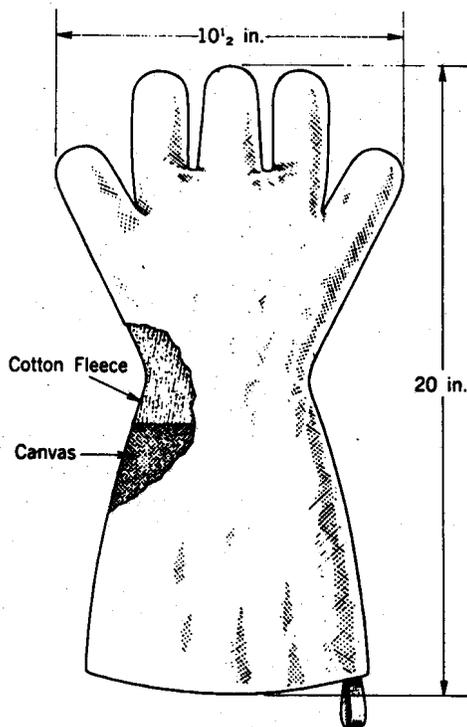
Fig. 7 - Asbestos Glove
